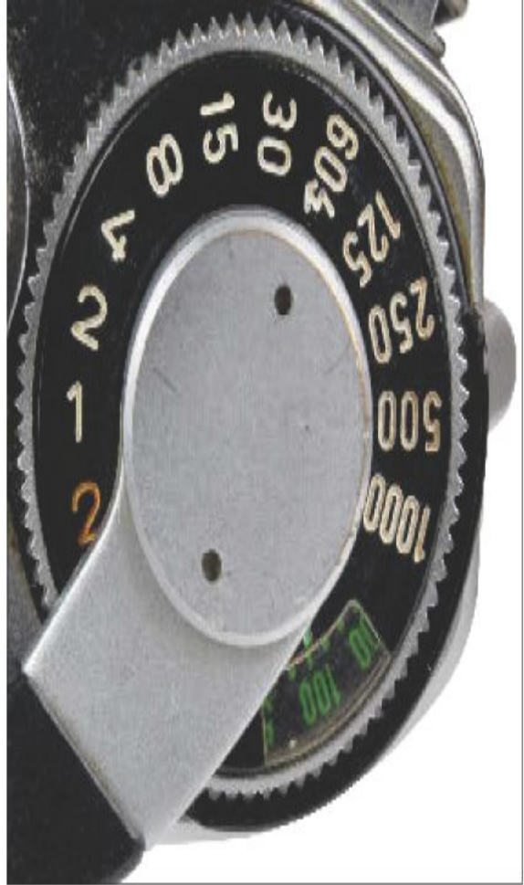
Shutter speeds are usually set on a camera's top plate dial. (Canon AE-1 shutter-priority camera)
